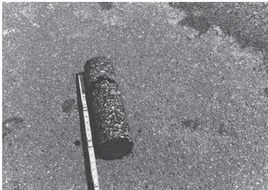
FIGURE 3.45 Core from flexible pavement indicating delamination about 3 in (75 mm) from surface.
