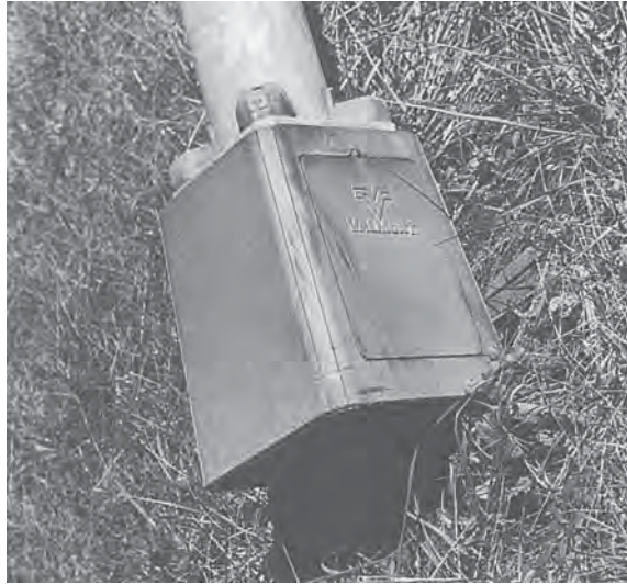
FIGURE 7.80 Separation of bottom flange from T-base.
