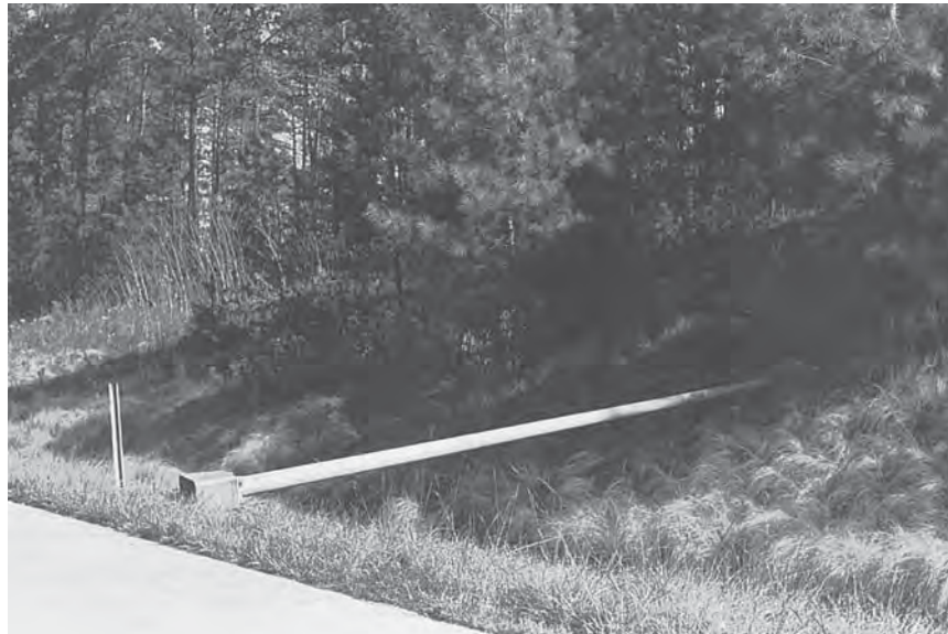
FIGURE 7.79 Failure of luminaire support without impact.
