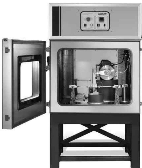
Figure 7.5 A two-point bending device on trapezoidal specimens. (Courtesy of Cooper Research Technology Ltd.)
