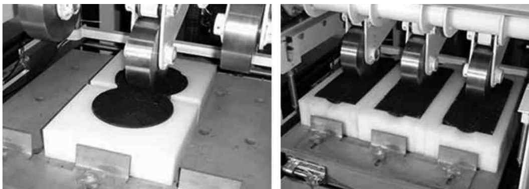
Figure 7.24 Specimens during the wheel-tracking test with the APA device. (Courtesy of Pavement Technology Inc.)
